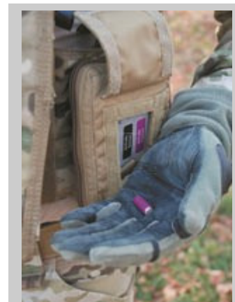
A wireless sensor is the second part of the BALSM system. When the warfighter ingests the capsule, the sensor within measures core body temperature.
